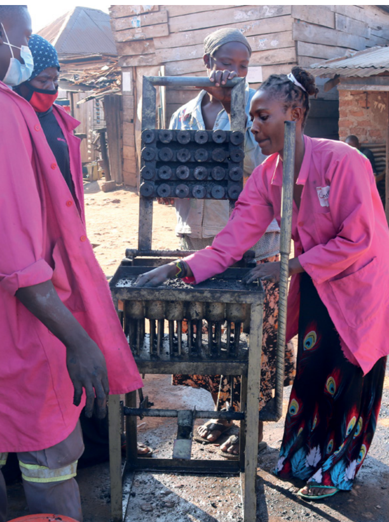
Members of the Kyosimba Onanya saving group demonstrating how to make briquettes (Left) Ready-made briquettes left to dry on a rack (right)
